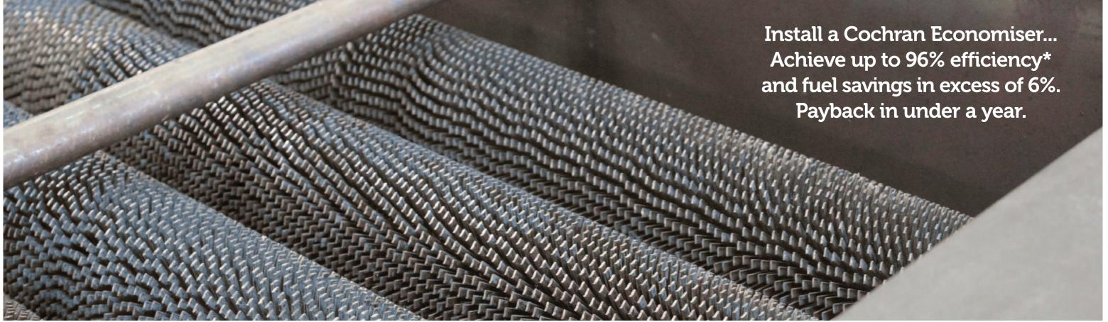
The use of an economiser can greatly reduce fuel consumption by utilising boiler flue gases to heat water for process services or to preheat boiler feedwater. Cochran design and manufacture economiser systems complete with all associated equipment to raise feed or returns water from a heating system.
